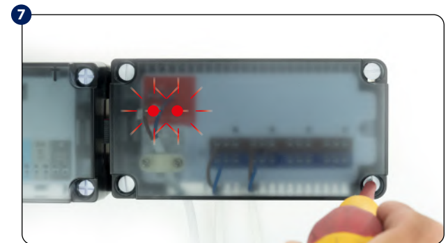
Make sure that all the wires are properly connected, mount top cover and power up the wiring centre - "Power" and "Connection" red LED diodes will light up indicating the correct connection with the KL08RF wiring centre.
